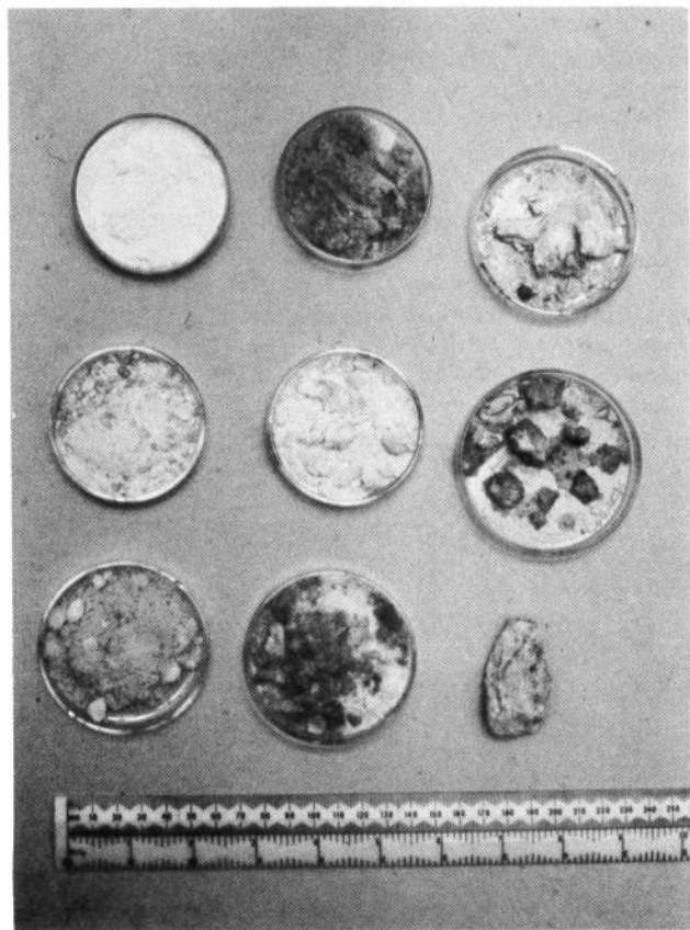
(8) Samples of natron and salt mixtures showing clumping and staining after use.
